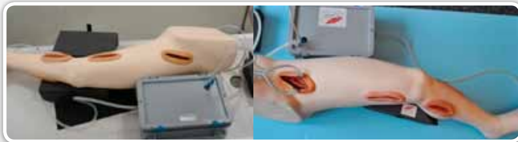
View of the new perfused leg model with waterpump and tube system
